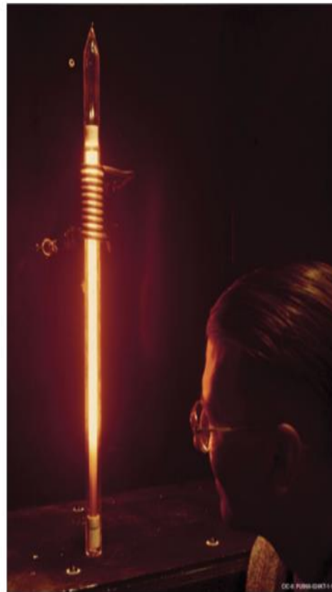
In this photo taken in the early 1960s, physicist George Grover tests a heat pipe.
